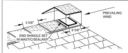
TRIM THE SEAL-DOWN END OF A RIDGEFLEX SHINGLE TO FIT AT THE END OF THE RIDGE, MAINTAINING THE EXPOSURE OF 5 5/8". SET STRIP IN MASTIC/SEALANT.
