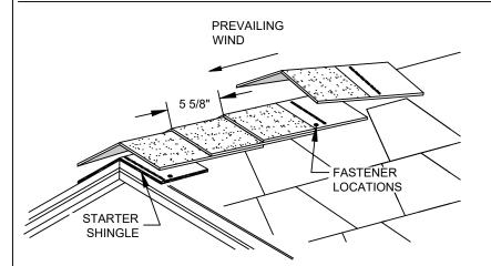
STARTER: CUT THE 5 5/8" EXPOSED PORTION OFF A RIDGEFLEX STRIP AND USE THE REMAINING SEAL-DOWN PORTION (7 5/8") AS A STARTER. POSITION WITH SEAL-DOWN AT ROOF'S EDGE, AND FASTEN 3" BACK FROM THE EDGE AND 1" UP FROM THE SIDE.
