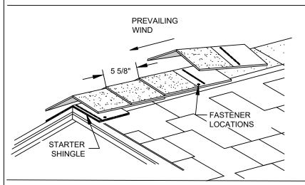
STARTER: CUT THE 5 5/8" EXPOSED PORTION OFF A RIDGEFLEX STRIP AND USE THE REMAINING SEAL-DOWN PORTION (7 5/8") AS A STARTER. POSITION WITH SEAL-DOWN AT ROOF'S EDGE, AND FASTEN 3" BACK FROM THE EDGE AND 1" UP FROM THE SIDE.
