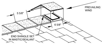
TRIM THE SEAL-DOWN END OF A RIDGEFLEX SHINGLE TO FIT AT THE END OF THE RIDGE, MAINTAINING THE EXPOSURE OF 5 5/8". SET STRIP IN MASTIC/SEALANT.
